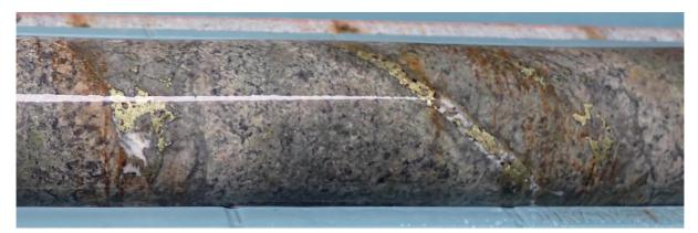
**Figure 6** – Silica-sericite altered, sheared granodiorite crosscut by quartz-carbonate- chalcopyrite veins (BRURD002: 201.4 – 201.7m)
