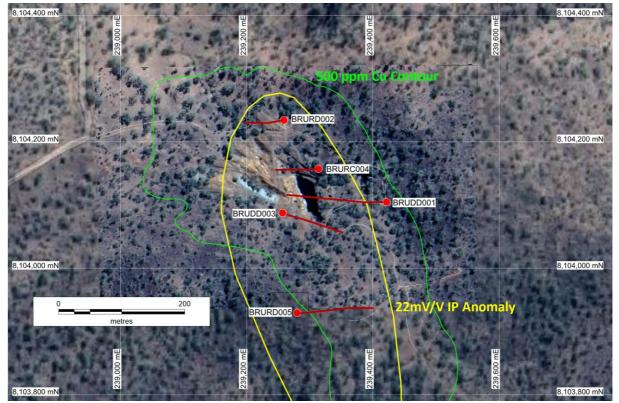
**Figure 5** – Plan view of Ruddygore area with location of +500ppm copper soil anomaly (green), 22mV/V IP anomaly outline (yellow) and the location of BMR drill holes drilled to date.
