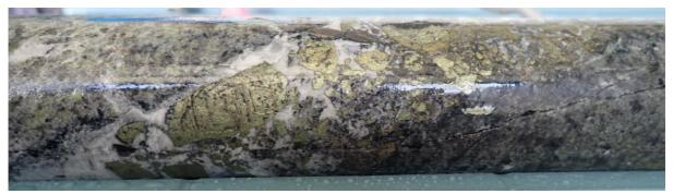
**Figure 7** – Silica-sericite altered, sheared granodiorite crosscut by quartz-carbonate-chalcopyrite veins (BRUDD003: 118.3 – 118.5m)
