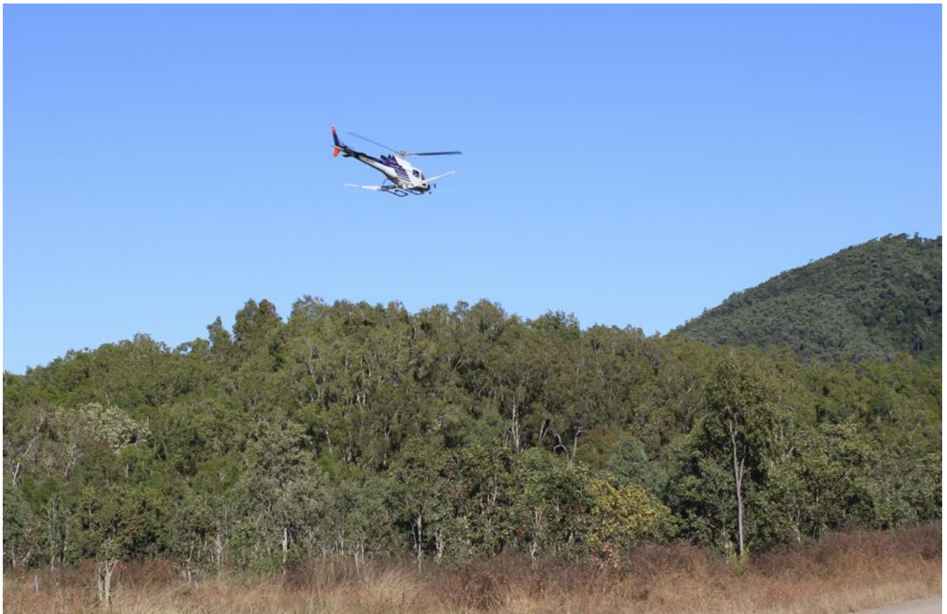
Figure 3. NRG's Xplorer™ heli-borne magnetic survey being flown over the Dittmer project area and funded by a Queensland State Government CEI grant.
