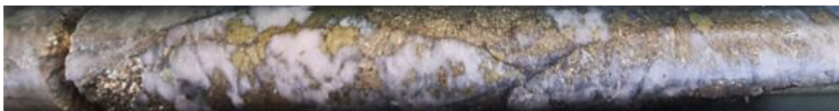
Figure 3. Drill core from drill Hole DTDD009 showing quartz-chalcopyrite vein material grading 171.8 g/t Au, 56.4 g/t Ag & 5.28% Cu
