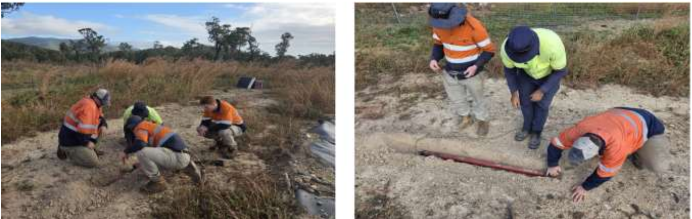
Figure 1 – Zonge field crew digging in sensors for the Dittmer MT survey.
