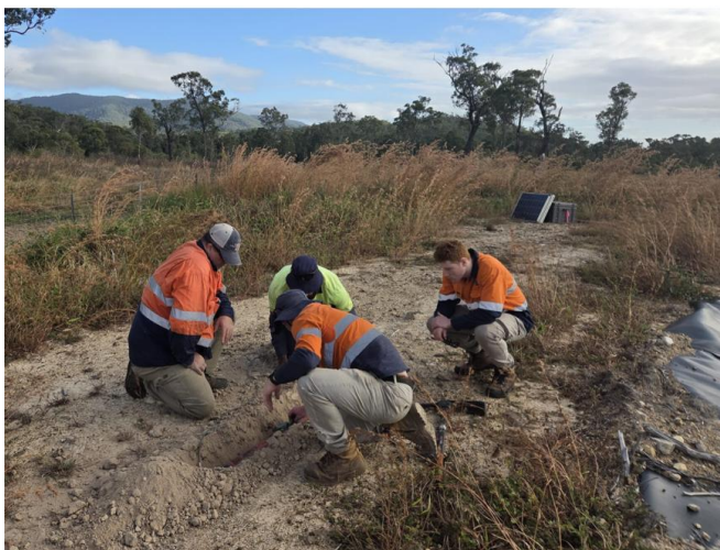
Figure 2 - Zonge field crew digging in sensors for the Dittmer MT survey.
