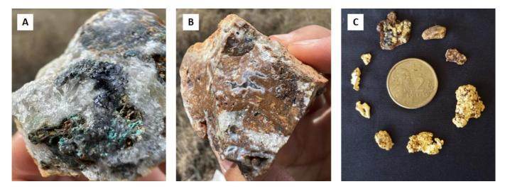
*Figure 1* – Recent samples from the Matthews Pinnacle area (A) Quartz-galena-malachite sample; (B) Ferruginous vuggy quartz sample; (C) Gold nuggets located in prospect area while mapping.
