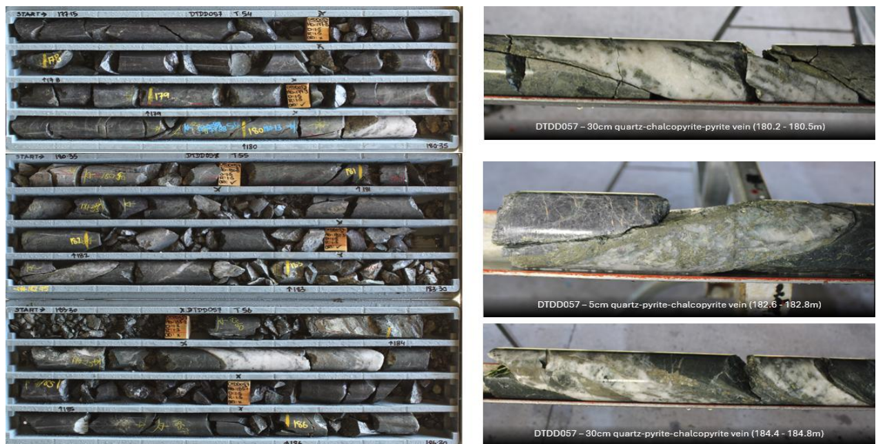
Figure 3 – Intersection of the Displaced Lode in DTDD057 including examples of quartz-pyrite-chalcopyrite veining.
