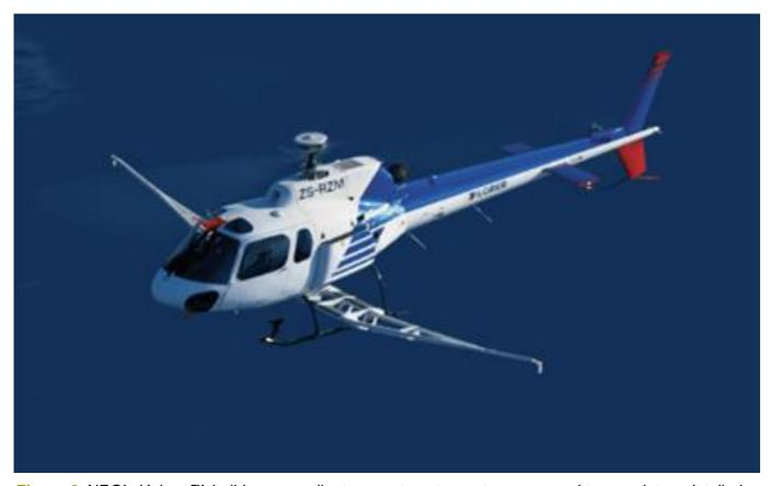
**Figure 6**. NRG's Xplorer™ heli-borne gradient magnetometer system proposed to complete a detailed magnetic survey over the Dittmer project area and funded by a Queensland State Government CEI grant.
