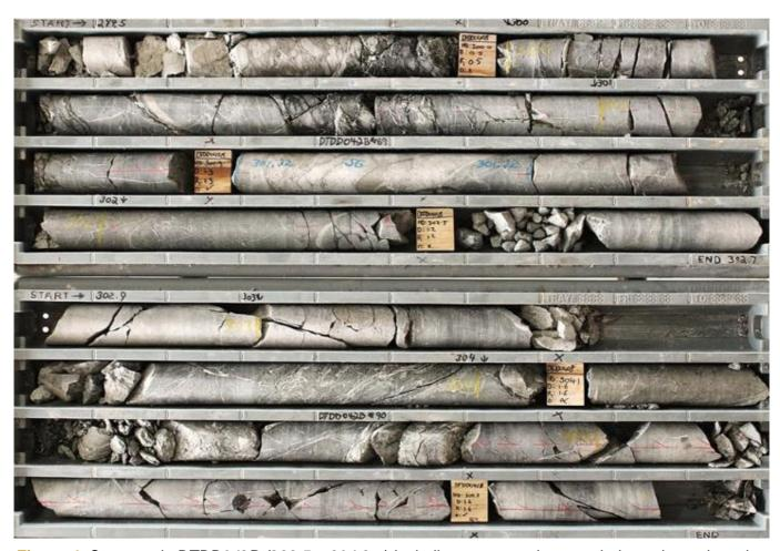
**Figure 4.** Ore zone in DTDD042B (299.5 – 304.3m) including quartz-carbonate-chalcopyrite-pyrite veins within sheared, silicified volcanics<sup>2</sup>.
