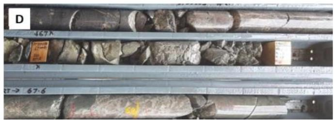
Figure 3 – (A) 10cm wide quartz-chalcopyrite-pyrite vein (DTDD030: 53.65 – 53.75m); (B) 30cm sheared quartz-pyrite vein (DTDD030: 86.9 – 87.2m); (C) Sheared and chlorite altered volcaniclastic rock overprinted by sheared 12cm quartz-pyrite-carbonate-chalcopyrite veins (DTDD031: 109.82 – 109.94m); (D) Faulted, brecciated volcanic overprinted by quartz-pyrite-chalcopyrite breccia zone (DTDD033: 67.8 – 68.2m).
