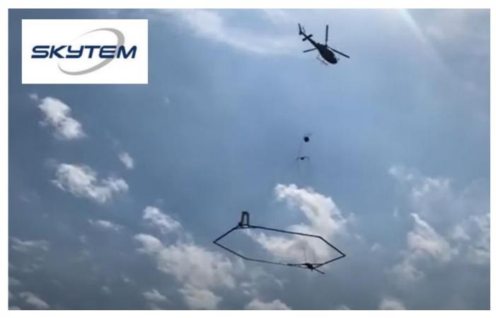
**Figure 7**. SkyTEM's low-frequency time domain EM and magnetic system. proposed to complete a detailed heli-borne EM survey over the Maniopota prospect (Ruddygore Project) and funded by a Queensland State Government CEI grant.
