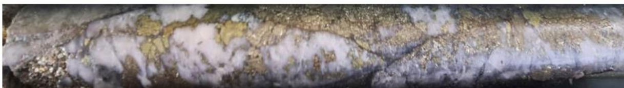
Figure 5. Drill core from drill hold DTDD009 showing quartz-chalcopyrite vein material grading 171.8g/t Au, 56.4 g/t Ag and 5.28% Cu
