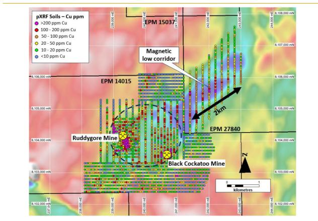
**Figure 1** – Ruddygore soil sampling showing pXRF results for copper (EPM 27840, Scardons); shown with previous BMR pXRF sampling (EPM14015), over RTP aeromagnetics.
