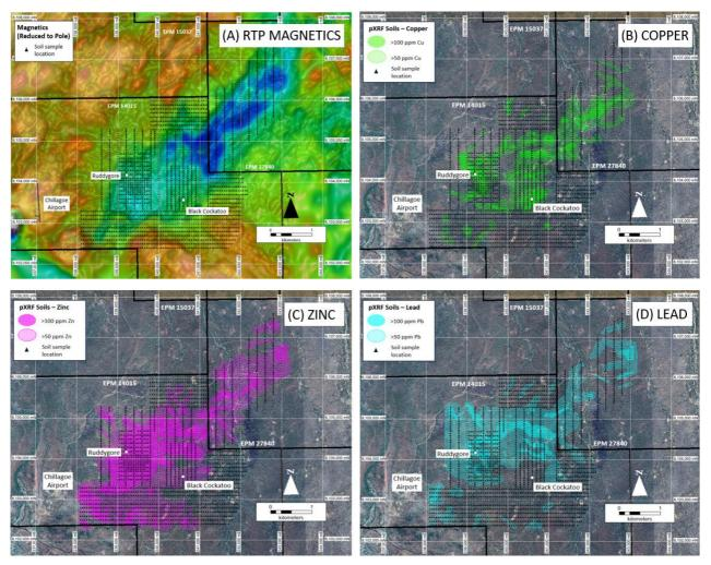
**Figure 2** – Ruddygore magnetic and soil results (A) Reduced to Pole magnetics image with soil sample locations; (B) Contoured pXRF copper-in-soil results; (C)Contoured pXRF zinc-in-soil results; (D)Contoured pXRF lead-in-soil results.
