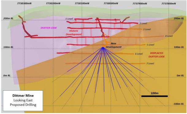
Figure 3 – Long section looking west at the historic Dittmer workings (red), displaced Duffer Lode (yellow) and planned initial drilling.
