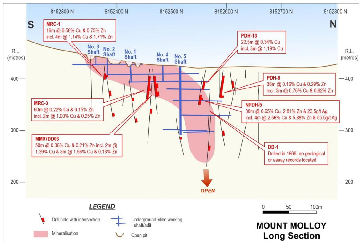
Figure 4 – Long section looking west at the Mount Molloy underground mine development, and historic drilling results.
