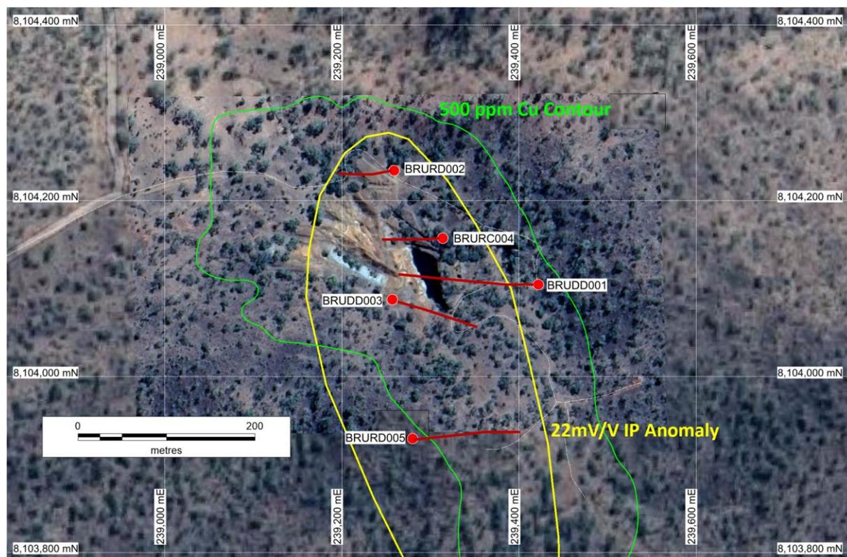
**Figure 5** – Plan view of Ruddygore area with location of +500ppm copper soil anomaly (green), 22mV/V IP anomaly outline (yellow) and the location of BMR drill holes drilled to date.
