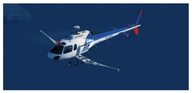
Figure 1- Example of an ASTAR B-series helicopter using the Xplorer<sup>™</sup> heli-borne gradient magnetometer system proposed to complete the survey.
