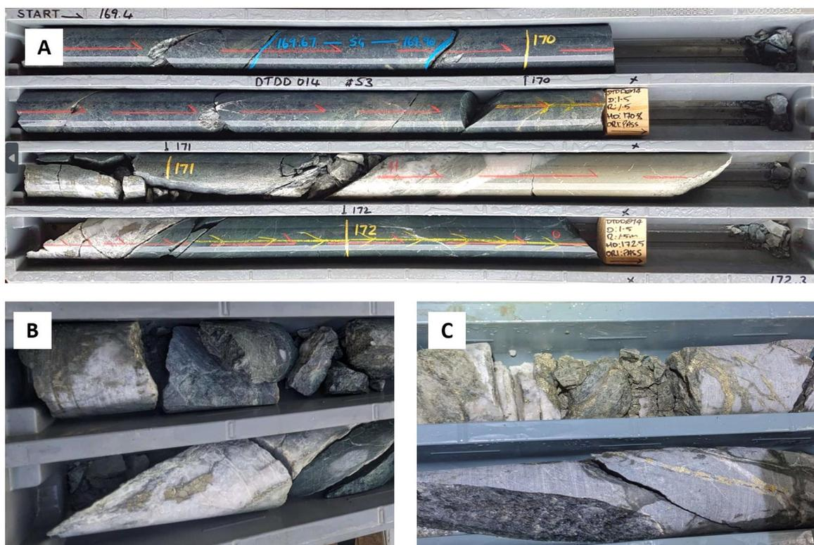
Figure 5 – Dittmer drill hole DTDD014 (A) core tray containing quartz-carbonate-pyrite-chalcopyrite veins (169.4 – 172.3m); (B) Close-up of 10cm quartz-pyrite-chalcopyrite vein (171.7 – 171.8m); (C) Close-up of quartz-pyrite-chalcopyrite vein stockwork (163.5 – 163.7m).
