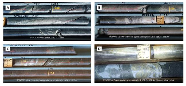
**Figure 5** – Examples of mineralisation encountered in recent Dittmer drilling (A) Pyritic shear zone in DTDD020 (232.3 – 232.9m); (B) Quartz-carbonate-pyrite-chalcopyrite veins in DTDD021 (165.5 – 168.0m); (C) Quartz-pyrite-chalcopyrite-carbonate vein in DTDD022 (102.0 – 102.2m); (D) Down-dip extension of mine lode in DTDD023A (167.7 – 167.8m).
