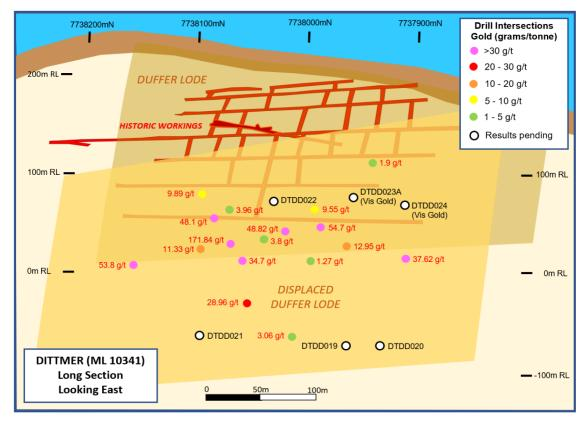
**Figure 4** – Long section looking east at the Dittmer Mine area, showing the extent of historic workings on the Duffer Lode as well as the location of the fault-displaced Duffer Lode and high grade gold drill intersections to date.
