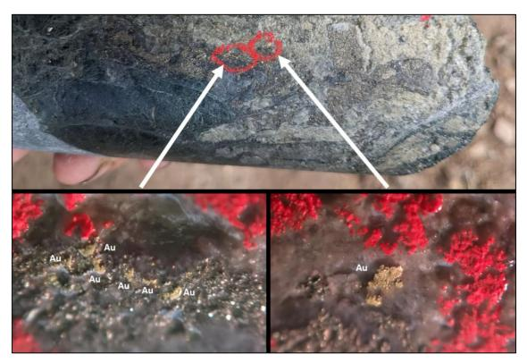
Figure 3 – Pyritic shear zone intersected in DTDD023A with visible gold (158.0 – 158.2m).
