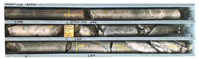
**Figure 2** – Dittmer drill hole DTDD015 core tray containing sheared volcanics overprinted by quartzpyrite-chalcopyrite veins (207.4 – 209.65m) with reported assay results of 2.25m @ 8.68 g/t Au, 2.8 g/t Ag & 0.25% Cu (207.4 – 209.65m), including 0.4m @ 37.62 g/t Au, 9.3 g/t Ag & 1.38% Cu (209.25 – 209.65m).
