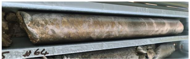
Figure 1 – Quartz-pyrite-chalcopyrite vein in drill hole DTDD015 (207.5 – 208.0m)
