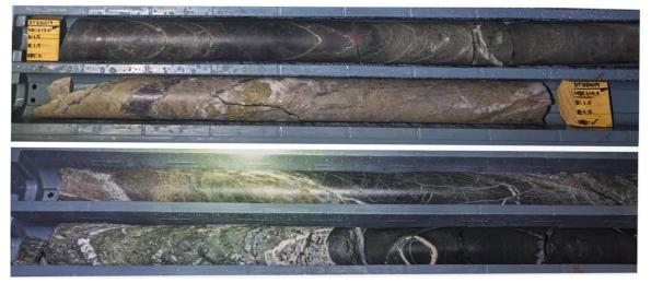
Figure 8. Dittmer drill hole DTDD019 core trays (213.0 – 216.2m) hosting andesite volcanics overprinted by pyrite-carbonate +/- chalcopyrite stringer veins (213.0 - 213.85m) and a variably sheared quartz-pyrite-chalcopyrite-carbonate stockwork zone (213.85 - 214.9m).
