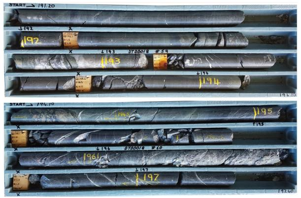
Figure 7. Dittmer drill hole DTDD018 core trays (191.2 - 197.6m) hosting andesite volcanics overprinted by a quartz-carbonate-pyrite-chalcopyrite vein (192.75 - 193.1m), a quartz-pyrite-chlorite fault breccia (194.1 - 194.4m) and a fault breccia and shear zone (195.8 - 196.65m).
