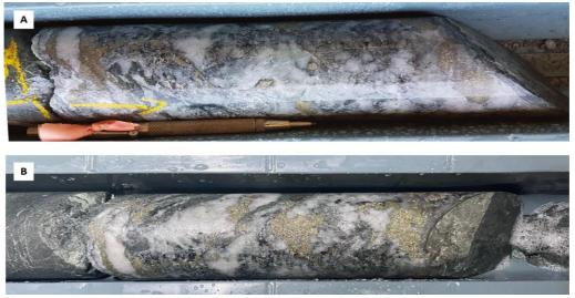
Figure 6 – Dittmer drill hole DTDD017 (A) Close-up of 20cm sheared quartz-carbonate-pyrite vein (166.37 – 166.65m); (B) Close-up of 20cm quartz-carbonate-pyrite vein (178.45 – 178.65m).
