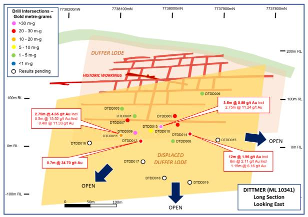
*Figure 3 – Long section looking east at the Dittmer mine area, showing the extent of historic workings on the Duffer Lode as well as the location of the fault-displaced Duffer Lode and location of drill intersections to date.*
