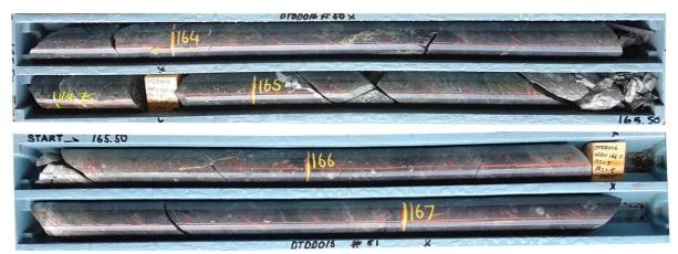
Figure 5 – Dittmer drill hole DTDD016 core trays containing quartz-sulphide veins (163.8 – 167.3m).
