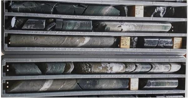
Figure 2 – Dittmer drill hole DTDD013 – andesite volcanics overprinted by a set of quartz-pyrite-chalcopyrite-carbonate veins (120.4 – 123.9m).
