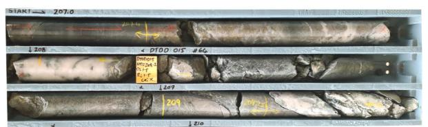
*Figure 4 – Dittmer drill hole DTDD015 core tray containing sheared volcanics overprinted by quartz- pyrite-chalcopyrite veins (207.4 – 209.6m).*
