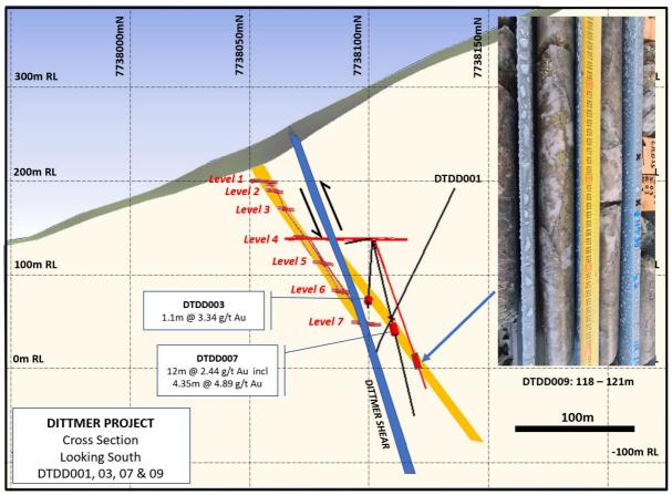
Figure 9 - Cross Section of Displaced Duffer Lode with Drilling and Underground Workings
