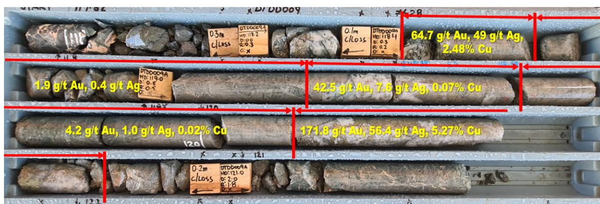
Figure 4 - DTDD009 HQ Drill Core Intersection of 2.25m @ 54.9 g/t Au, 20.6 g/t Ag & 1.52% Cu from 118.4m. This intersection is typical of the mineralisation observed in the historic Dittmer Mine.
