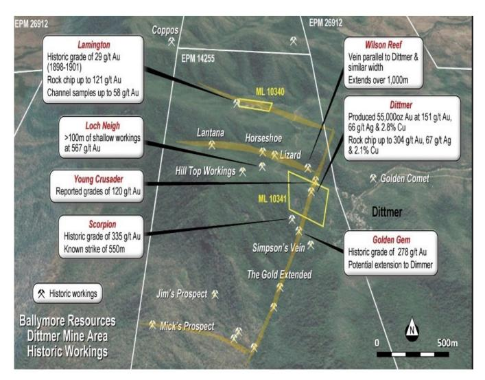
Figure 2 – Historic mine workings and interpreted structural corridors in the Dittmer area.
