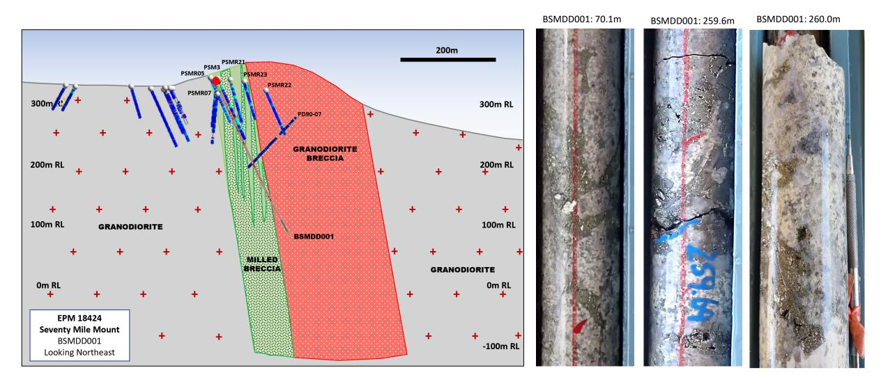
Drill hole BSMDD001 completed at 351.04m and intersected broad zone of milled and crackle breccia
