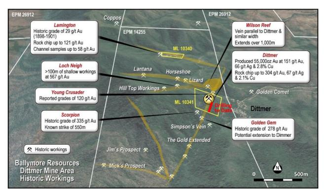
Figure 4 – Historic mine workings and interpreted structural corridors in the Dittmer mine area.
