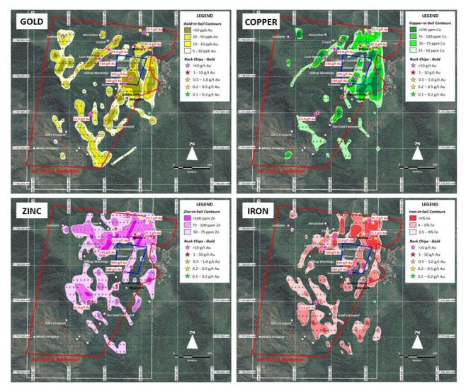
Figure 3 – Dittmer area contoured soil results including gold, copper, zinc and iron.
